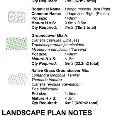
This plan should be read in conjunction with the architectural and hydraulics plans. Work specific to these plans should be prepared in accordance to these plans, including specification and details prior to the installation of landscaping, and should not be altered or compromised during landscape construction. Retaining wall details to engineers design. Elements such as drainage swales may be incorporated in garden bed areas (using non-floatable mulch) without compromising the capacity or form.
